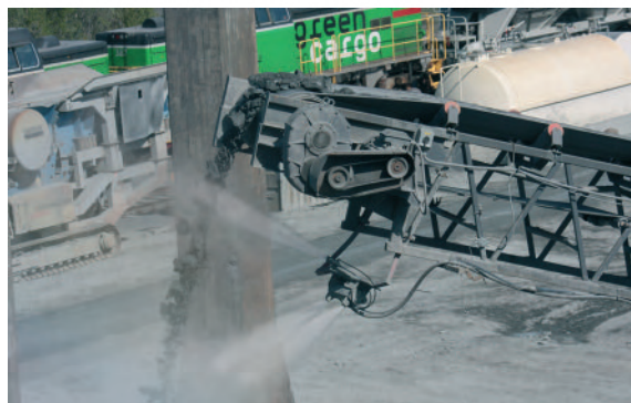
PZ series air-atomizing nozzles at a conveyor belt discharge
