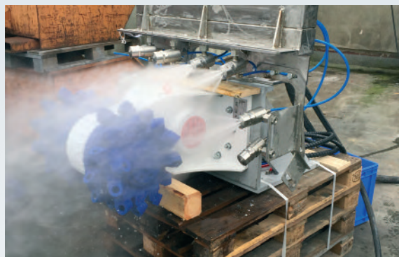
Internal spray testing to optimize nozzle configuration
